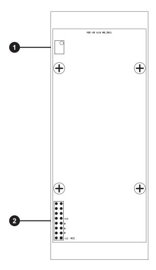
1 CALIBRATION POINT: Removes DC offset at both outputs. Factory calibrated to 0V DC (*Please see 'CALIBRATION' on page 7 of this guide*)
