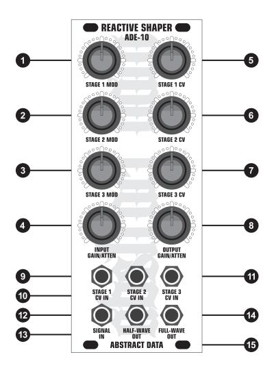
1 STAGE 1 MOD: Vertical waveshaping for subtle phasing and PWM-style effects
