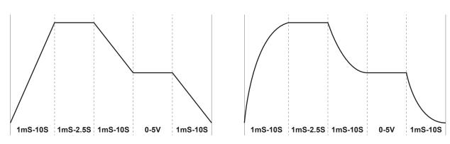
Linear envelope response is characterised by smooth, even rise and fall times and Exponential envelope response is characterised by a curved response that 'speeds up' over time.
