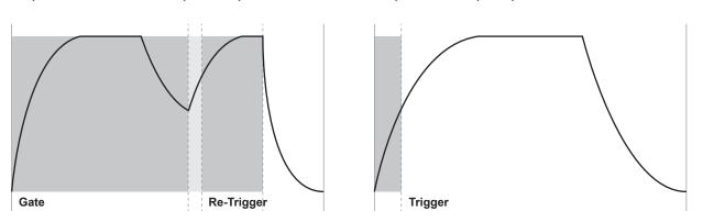
The AHDSR envelope type can be re-Triggered at any stage after Hold. The envelope stages start again from the Attack stage at whatever level the envelope it is at when re-Triggered. When the initial Gate signal ends - the envelope enters the Release stage as normal. The AHD envelope type operates independently of Trigger/Gate length with all stage times set by the relative front panel controls.
