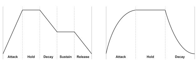
AHDSR is the ADE-51s standard, 5-stage envelope type, generated by a gate signal. A 3-stage AHD envelope can also be generated using the Trigger input where the time of the total envelope is set by the length of each stage and is independent of the Trigger/Gate length.
